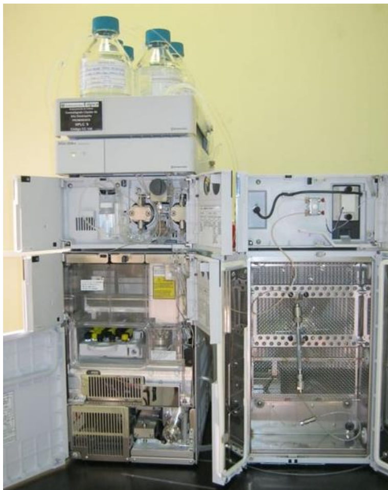
Figura N°5 Interior del HPLC Prominence LC-20AD
