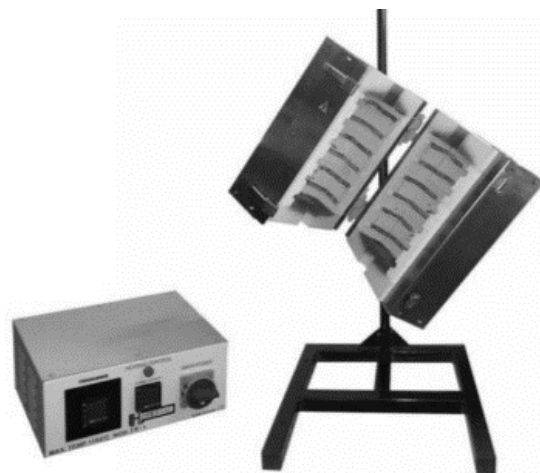
Fig. 2.3. Horno tubular vertical de alta [23].
