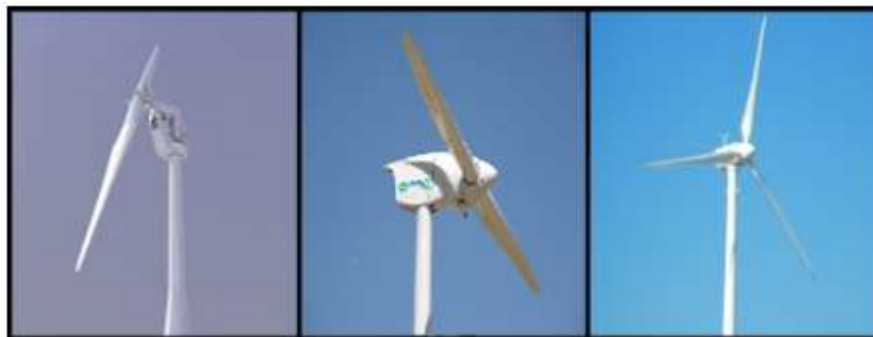
Figura 2.2 – Aerogeneradores monopala, bipala, y tripala (Renovetec, 2019)(3)
