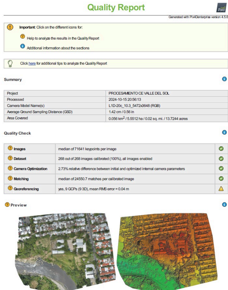
Figure 1: Orthomosaic and the corresponding sparse Digital Surface Model (DSM) before densification.
